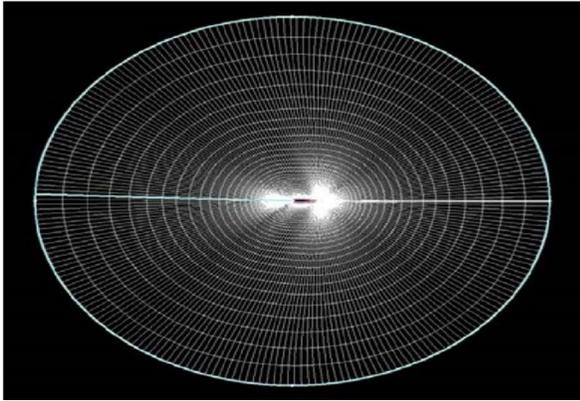
**FIGURE 1:** STRUCTURED O GRID ON ADE AIRFOIL
