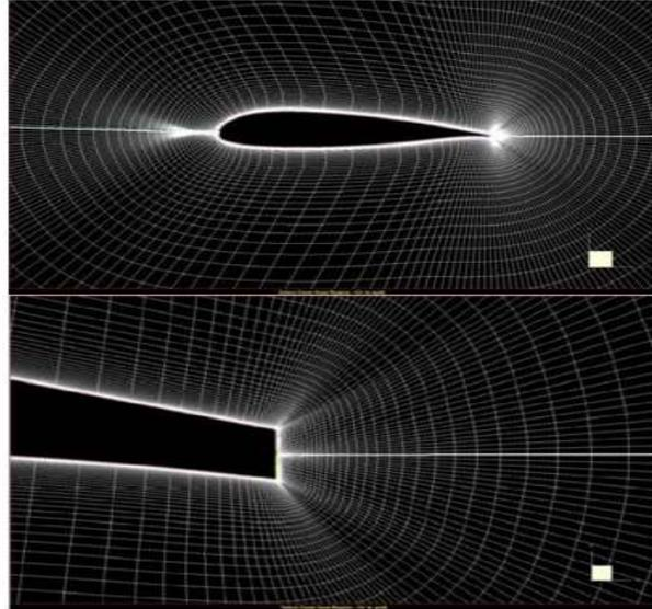
**FIGURE 1c:** ENLARGED VIEW MESH-2 TRAILING EDGE REFINEMENT AT BOTH END & MID POINT
