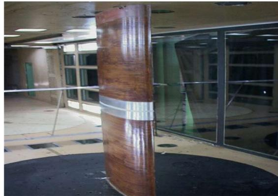
FIGURE 11: ADE AIRFOIL MODEL ON THE SYNCHRONOUSLY DRIVEN TWIN-TURNTABLES (FLOOR AND ROOF) AT NWF, IITK.
