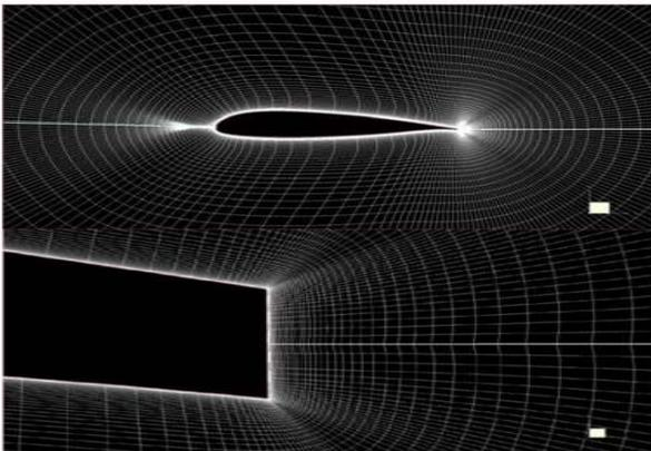
**FIGURE 1b:** ENLARGED VIEW MESH-2 TRAILING EDGE REFINEMENT ONLY AT BOTH END
