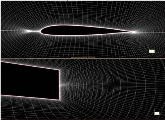
**FIGURE 1a:** ENLARGED VIEW MESH-1 WITHOUT TRAILING EDGE REFINEMENT
